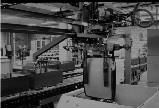
Fig. 1. Television set assembly: an example of a MATS manufacturing system (courtesy of Philips Electronics, Eindhoven, the Netherlands)
